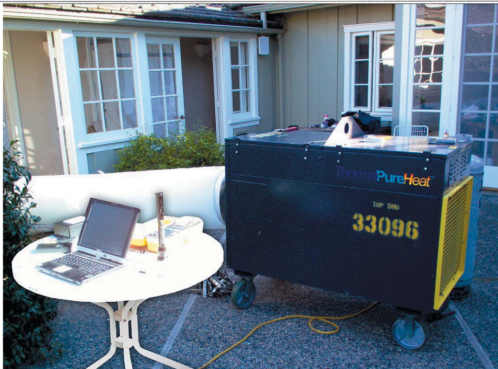
Mold remediation contractors use this propane heater in conjunction with air blowers to inject superheated air into moldy homes. Company official tout this as an effective chemical-free way of ridding a home of mold infestation.
